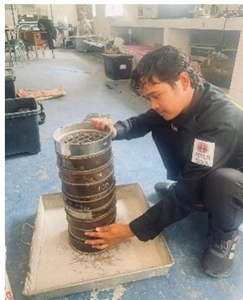
Figure 1. Aggregate Gradation Testing Process
